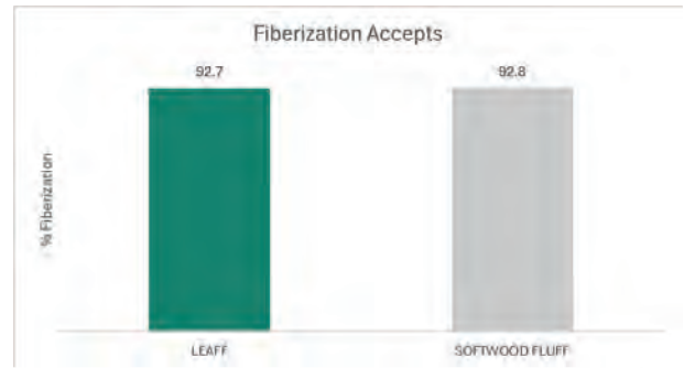
Comparison of fibreisation quality between Leaff and softwood fluff
