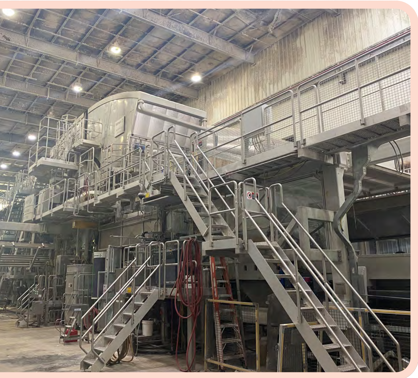
ST Paper's Barnwell County-based plant: the acquisition included a 30,000tpy Valmet-supplied hybrid QRT/DCT TM
