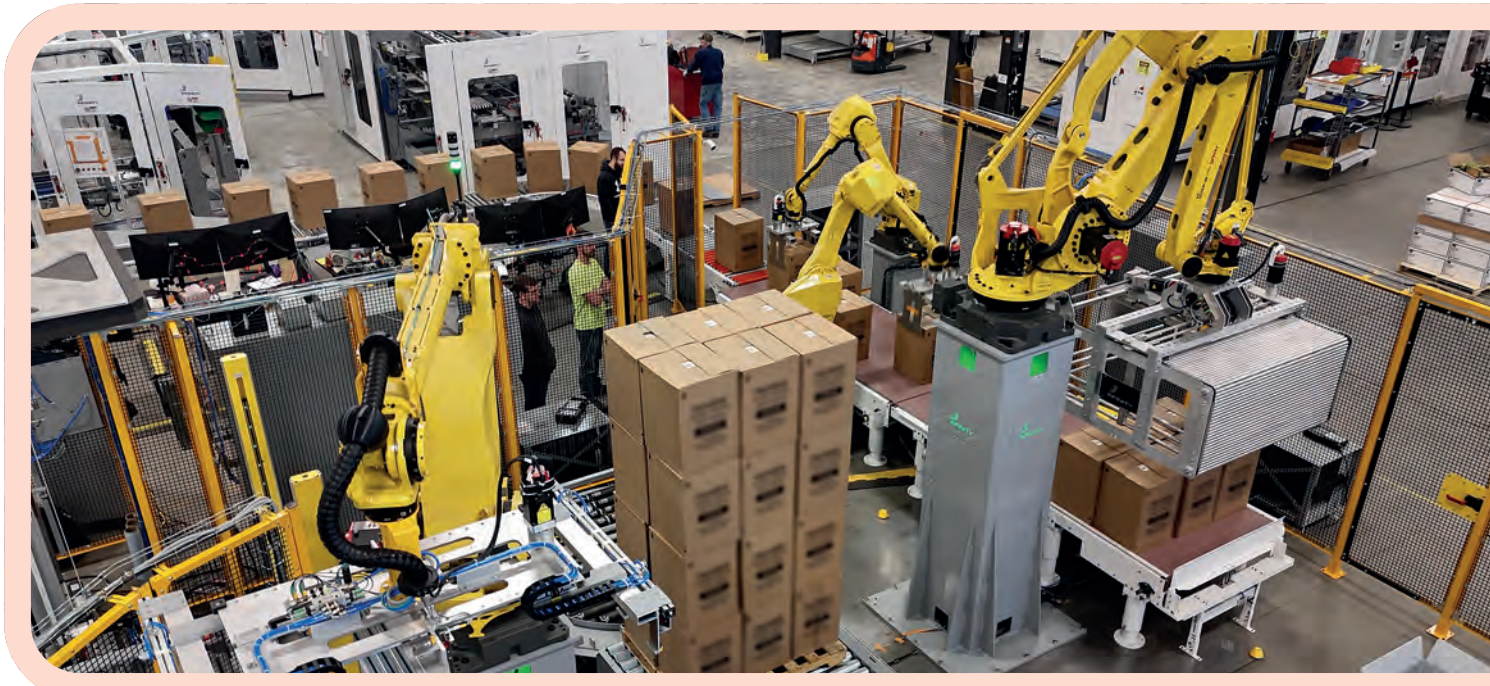
High throughput applications: Infinity palletisers can be equipped with multiple sorting arms, loading arms and build station
