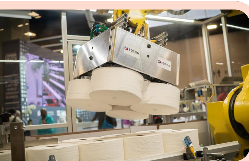
Flexibility, space efficiency, and modularity: the Edson 4000TL is designed for delicate or irregularly shaped items
