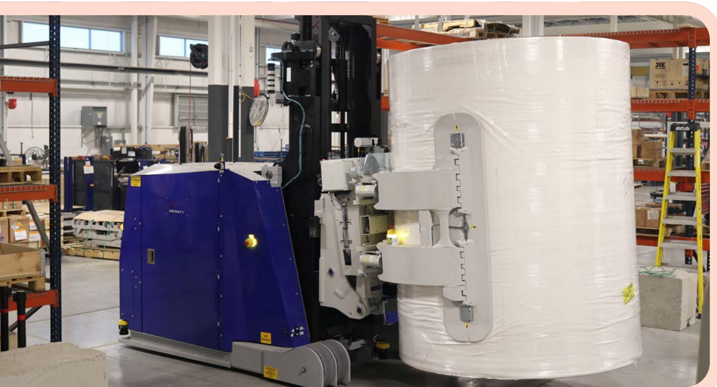
The CB39RC, one of Infinity's AGVs: a counterbalanced vehicle with a fully articulated clamp arm that boasts a 3,900kg lifting capacity
