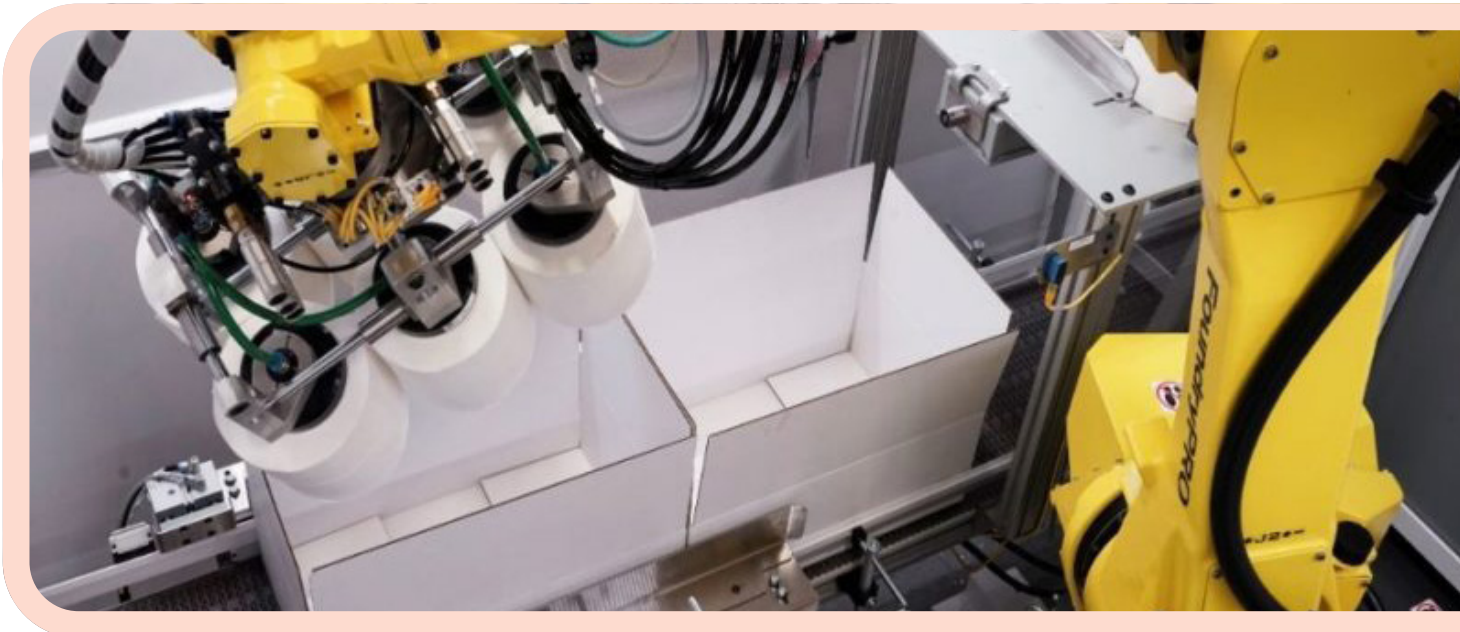
Reliability and precision: the Edson 4000TL packing toilet paper rolls into cases
