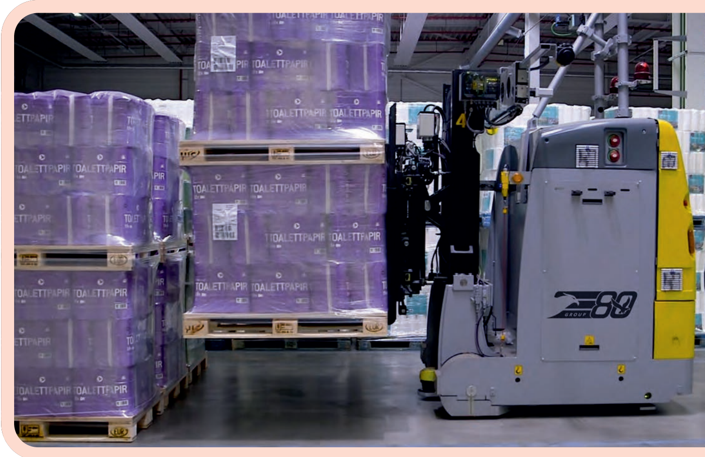
Finished Goods Block Storage System with LGVs.
