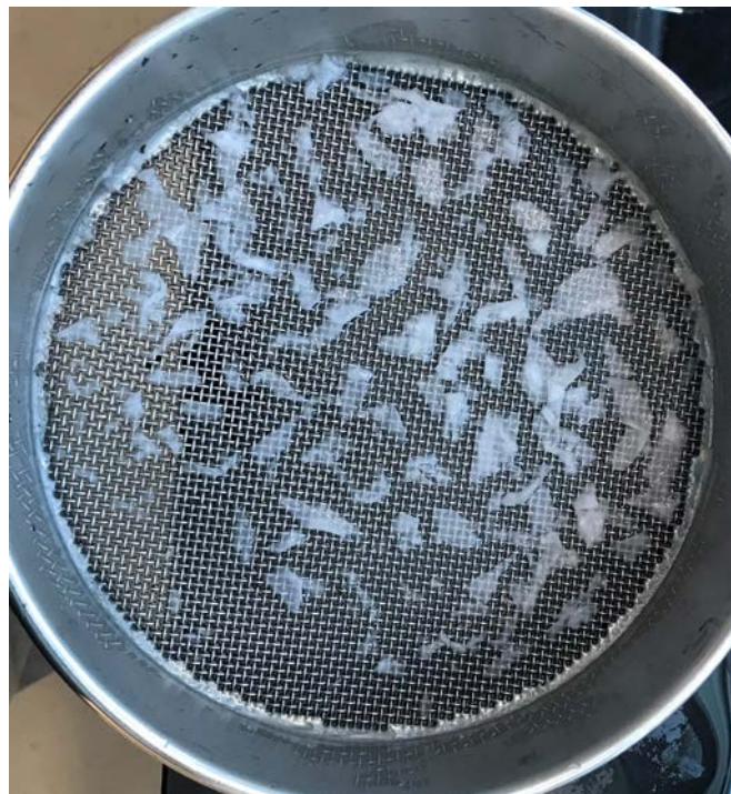
Figure 6: Picture of the sieve after screening the repulped handsheets made with PAE resin.
