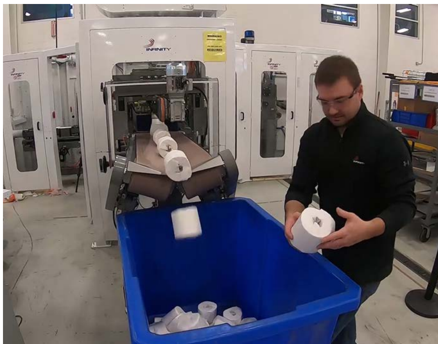
Innovative ecological packaging: The C15 Casepacker is capable of loading rolls into corrugated trays, providing stable secondary packaging for tissue products
