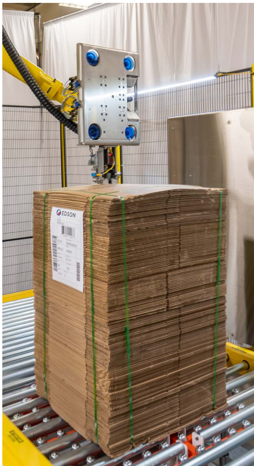
A point on cleanliness: This system safely chops the bands into a bin for better waste management
