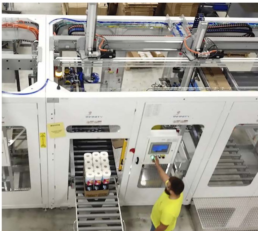
Cuts down on material waste: The C15 can also package large-roll-towel directly into corrugated cases without the need for additional packaging
