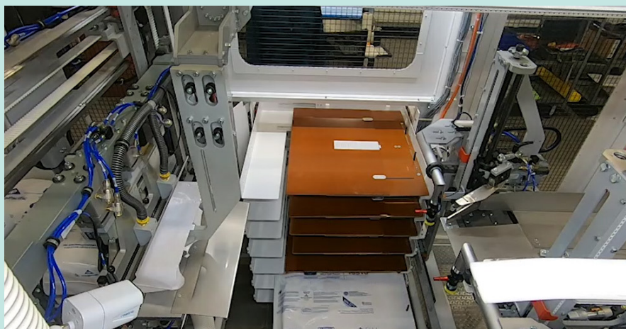
The new multi-shelf wicket system: seven shelves can each be filled up to two inches high with poly bags
