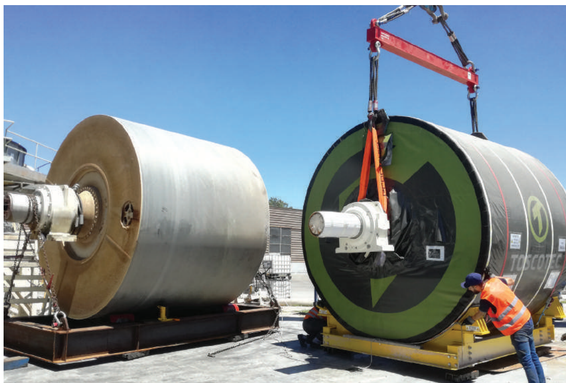
Latin American capacity boost: CMPC's new TT SYD-12FT has a diameter of 3.6m and a width of 2.8m.
