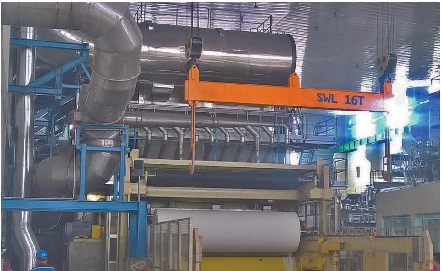
Reaching new heights: APP's new 22 ft Steel Yankee dryer is said to be the biggest ever manufactured for tissue
