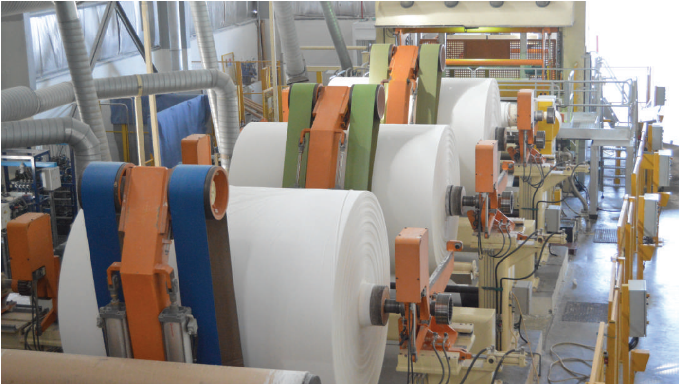
Product variety: from its 50,000sqm plant, CPM produces jumbo rolls for a variety of products, from 13.5gsm facial tissue to 45gsm hand towels, all from high-quality virgin pulp grades.
