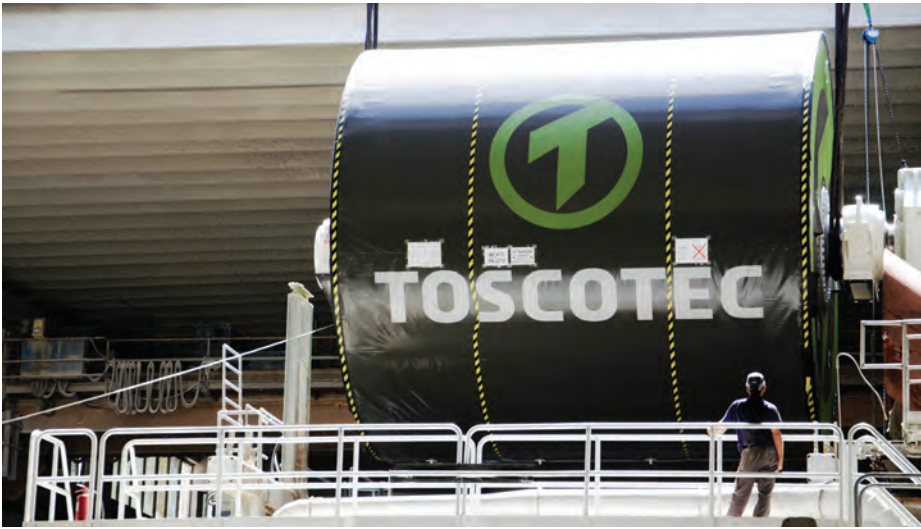
Above: The 5,600mm wide machine is said to be Europe's largest Steel Yankee Dryer for tissue production
