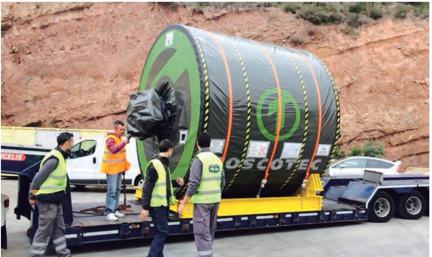
Delivery at ISMA 2000's La Torre de Claramunt mill included a Steel Yankee Dryer TT SYD-3,600mm
