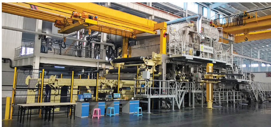
The AHEAD-1.5m tissue machines will increase Vinda's production capacity by 60,000tpy
