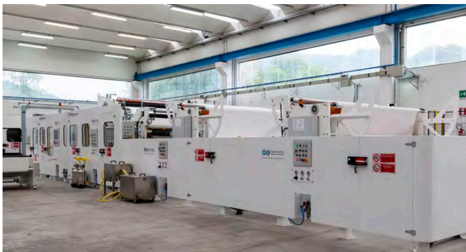
Lamix's Amica Matrix industrial line converts industrial laminated rolls at a speed of 550mpm
