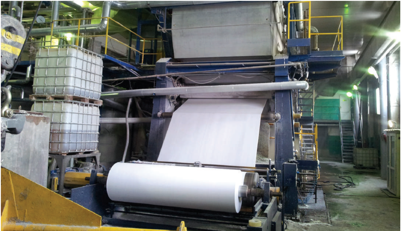
In 2004, Karina purchased PM2, a 2.3m working width former kraft paper machine of Italian origin
