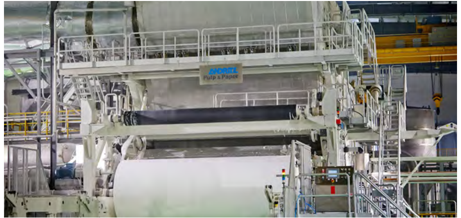
PM27 has a width of 5,62m and a design speed of 2,000m/min. Next year, an identical machine is also scheduled to start production
