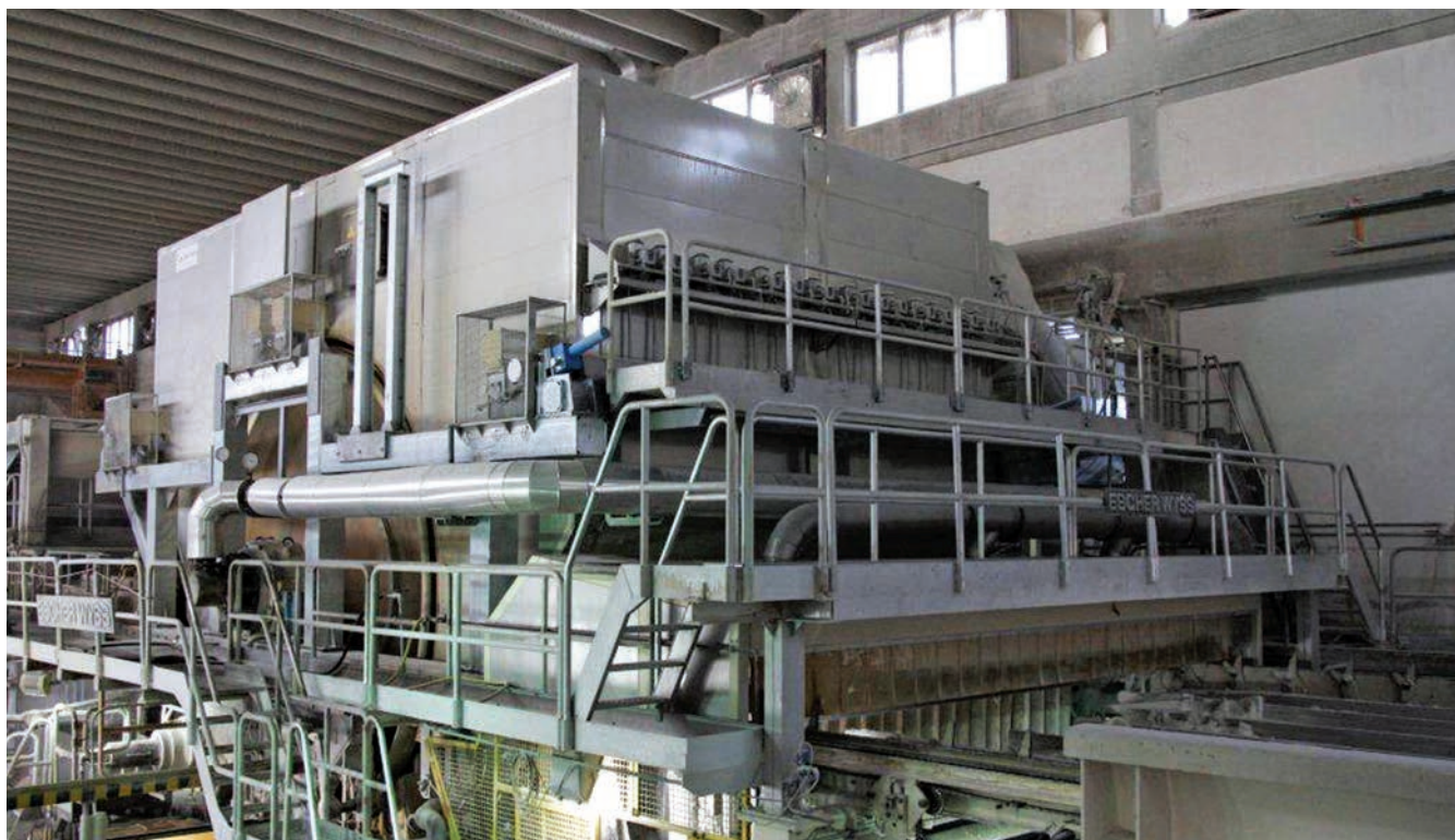
The new hood at Wepa has reduced gas consumption by more than 20%
