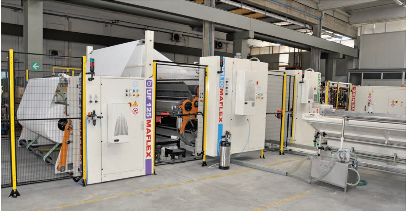
Maflex's continuous and fully automatic ARES line is able to produce both AfH and consumer rolls.
