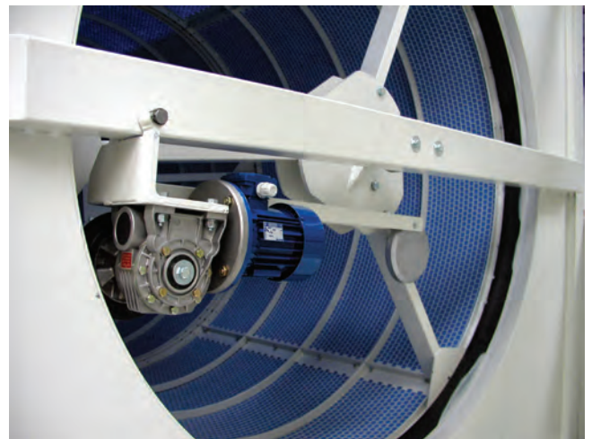
Inside the multi waste filter; the point where the filtered air exits from the self-cleaning filter
