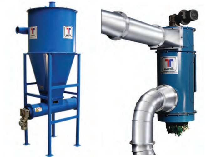
Typical devices used to discharge the collected dust. On the left is the cyclone separator with final horizontal screw conveyor. The second is a vertical compactor where the screw conveyor is inside in a vertical position.
