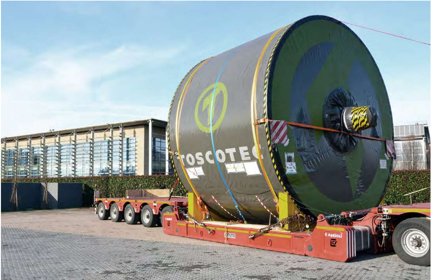
Oji Group's new TT SYD has a diameter of 12ft and a face length of 5,750mm
