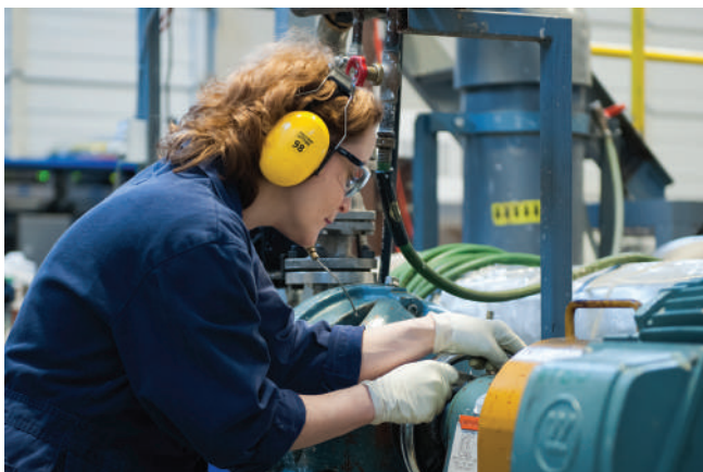
Figure 4: Canfor Pulp Innovation tests all pulps using a 12" Sprout Bauer refiner to ensure data relevance to customers which cannot be obtained by PFI beating alone
