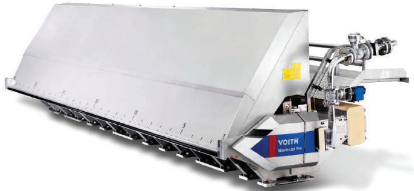
"Excellent quality level": The MasterJet Pro T headbox
