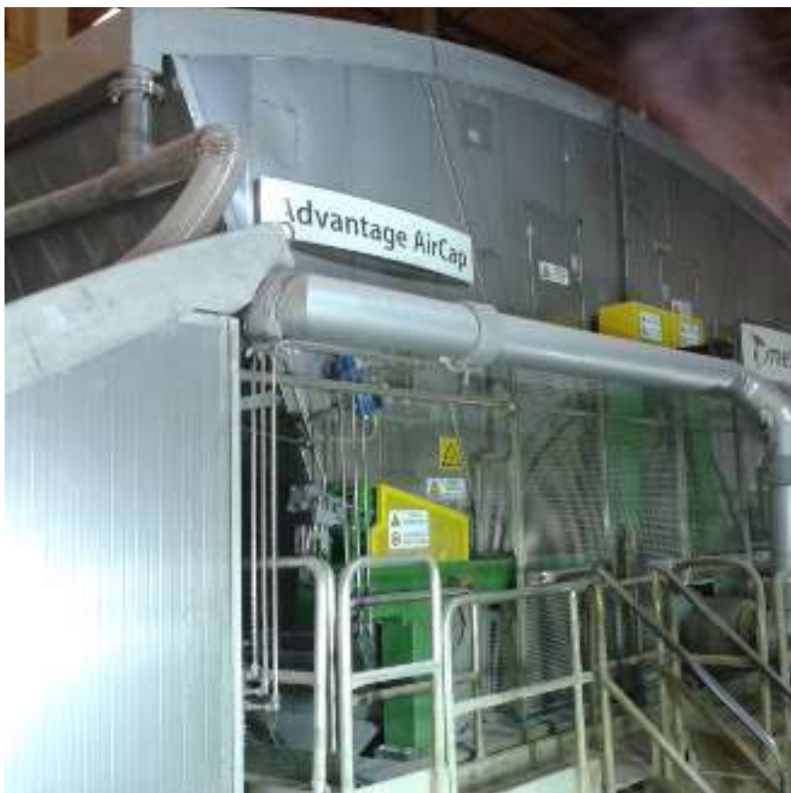
The Yankee Advantage AirCap hood and Advantage WetDust dust control system at UK-based Disley Tissue
