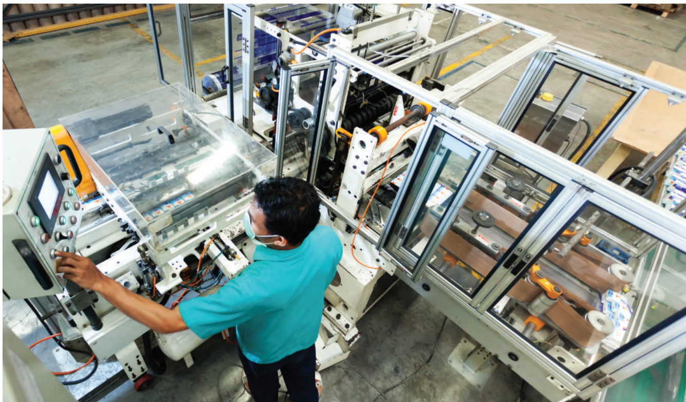
One of the converting units in Pindo Deli 2. The mill has 57 converting units for tissue rolls, folded tissue, towels and packaging. 80% of the Jumbo Rolls produced by the mills tissue machine is converted internally on site.
