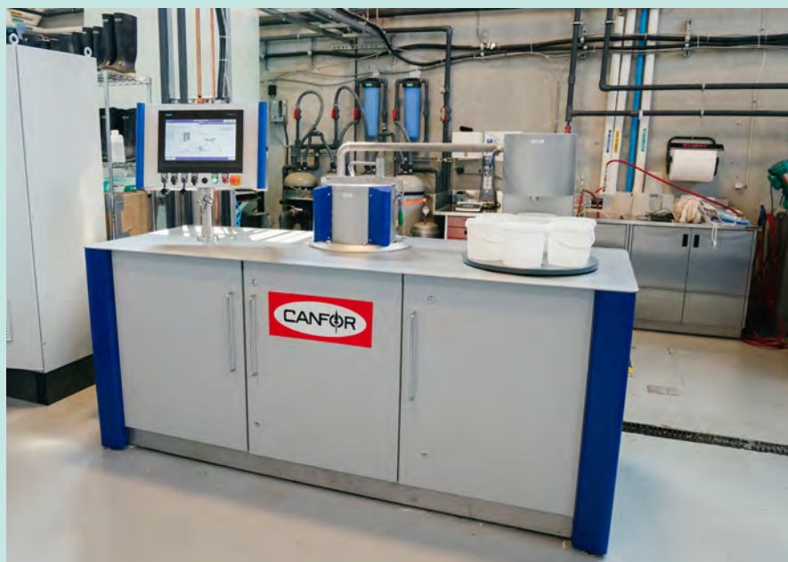
Fig 1: CPI's LR40- lab disk refiner a versatile, accurate pilot instrument provides refining information that is applicable to mill scale.
