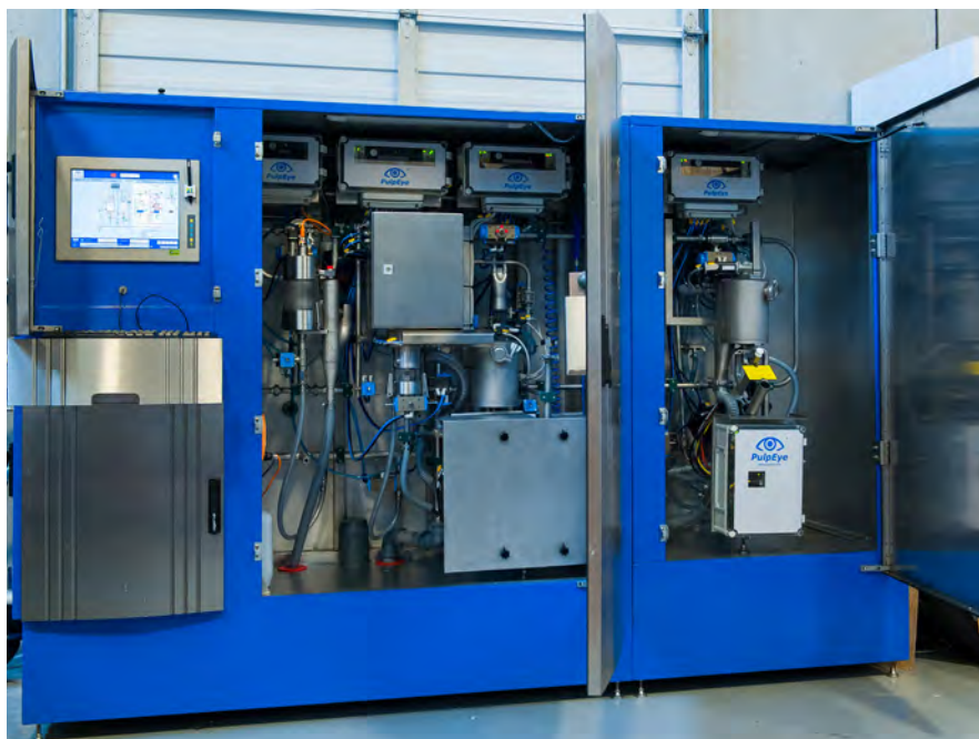
Fig 2: CPI's PulpEye used for rapid assessment of pulp and fibre properties such fibre length, fibre width, coarseness, kink and curl. Each kraft fibre line has a PulpEye providing real time data.
